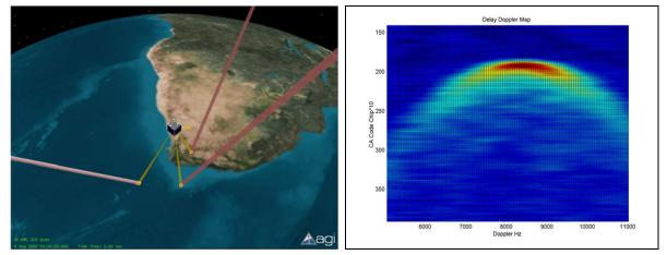
An example reflection is shown on the right in the figure above for a signal detected off the ocean. The x-axis shows the frequency response of the reflected signal and the y axis shows the spreading in delay. The rougher the surface the more spreading appears in the received signal in both directions [4].
